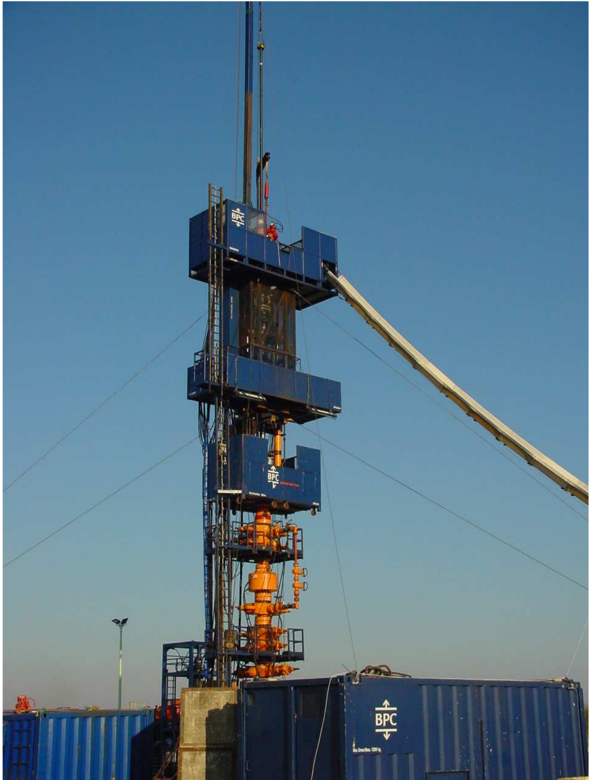
385k Space Saver II during a Snubbing operation
