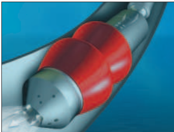
Unique tool design provides jetting action ahead of the thruster.
